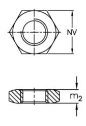
$\begin{array}{ll} m2 &= 7.0\\ Nominal size = M14\\ NV &= 22.00\\ Thread pitch = 2.00\\ Weight (g) &= 15.0 \end{array}$
